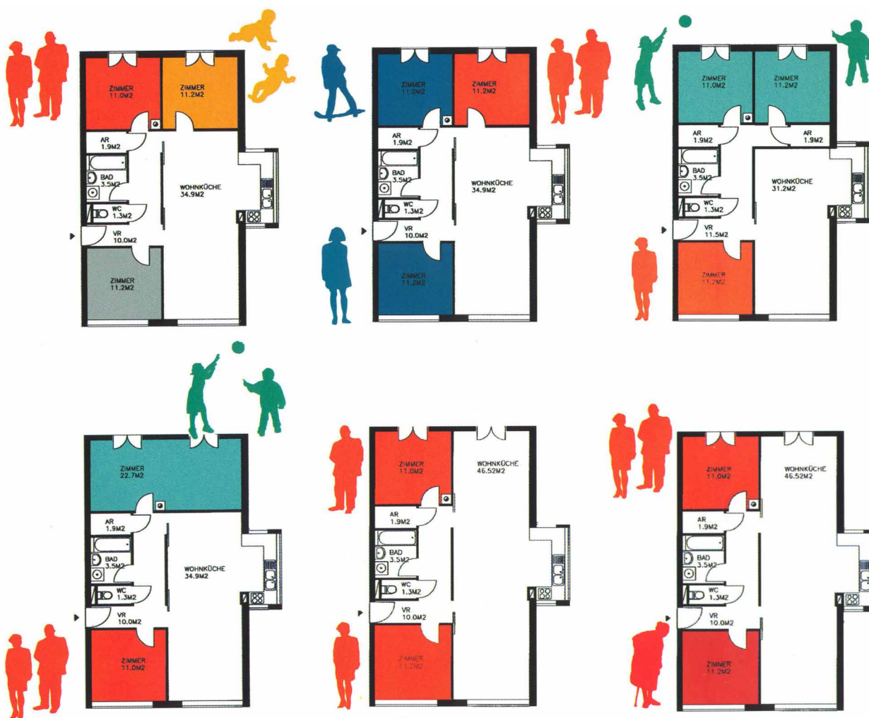
Figure 2: Flexible apartment layouts that are 'use neutral' and can be adapted to the specific needs of the household
